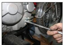
2) Remove the oil drain plug to drain the engine oil
