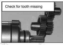
3) Check the idle gear shaft and Starting dual gear shaft for
