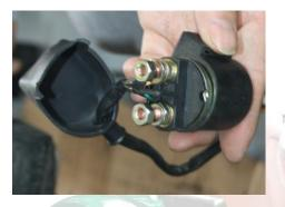
13. Check clutch electrical starting switch plug whether is
