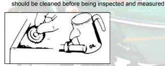
To clean the spare parts, use only the cleaning fluid that is incombustible or has high ignition point. Before reassembling, apply the specified lubricating oil to the sliding surface of the parts and components. After reassembling, check whether all the spare parts are mounted properly by means of turning, moving and
