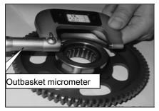
7) Measure the washer thickness, the maintenance limit:  $\geq$
