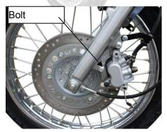
Operating brake, if the wears limit line of the brake shoe touch to the basket of the brake disc. It shows that the brake shoe has touched the wear limit. \_\_\_\_\_Front wheel, front overhang and steering stem **Replace the brake shores.**
