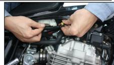
8. Pull off the fuel level sensors control wire patch plug.
