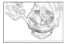
Measure the piston pin external diameter.
