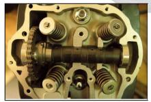
3) Remove the camshaft end cover, loosen the screw and washer at the tail end of the tensioner; turn the screw clockwise with the tensioner locking key so that the tensioner is loosened and locked.
