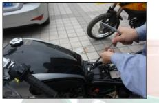
5. Loosen the tube clamp and pull off the fuel tube
