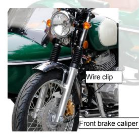
Unscrew the upper / lower connection plate bolt and. the direction of the tube bolt
