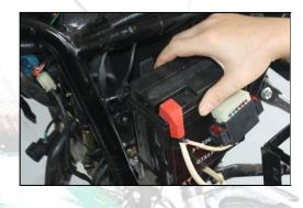
7. check connector socket of rectifier and measure output
