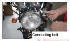
Remove the 2 connecting screw in the front face of
