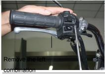
• Loosen the retaining bolt and remove the clutch handle
