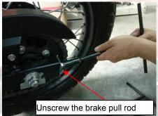
4) Dismantle rear wheel axle nut to check it whether is
