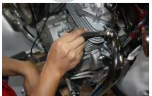
2) Remove the engine cycle tube
