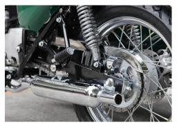
Unscrew the rear wheel nuts、 the brake pull rod、 Brake limit lever and remove the rear wheel spindle.
