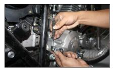
10. Remove the starting motor wire.
