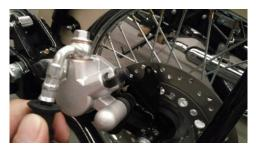
Don't touch brake pedal when you disassemble caliper
