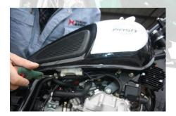
6. Pull off the fuel pump relay control wire patch plug.
