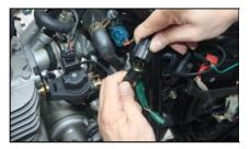
16. Remove the inlet pipe connected to the engine bolt
