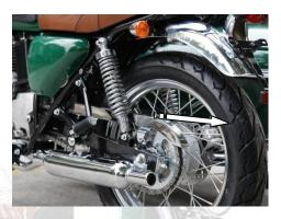
Installation of rear wheel Installation is in the reverse order of removal. While mounting the rear wheel, make sure the spindle bushes on both baskets are aligned and the brake caliper clamps the rear wheel hub. While installing, properly adjust the chain adjuster to ensure that the chain slack is between 15mm and 25mm and that the left and right scale lines of the chain adjuster are consistent, and then fasten the rear wheel spindle nut to the required tightening torque of 50-60N.m
