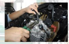
7. Remove Left /Right cylinder head connecting pipe
