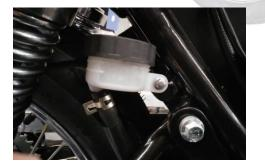
If the brake lever feels mushy when pulled, there may be air in the brake lines or the brake may be defective. Since it is dangerous to operate the motorcycle under such conditions, have the brake system immediately checked
