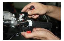
12. Check switch plug of relay whether is loose.
