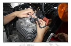
5) Unclamp the inlet pipe clip and remove the cylinder head hanging bolt.
