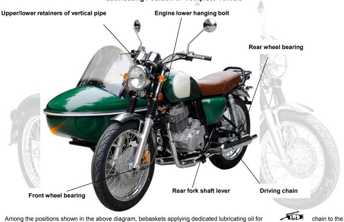
driving chain, apply lithium base grease to all other positions.
