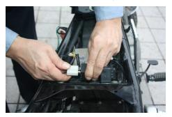
7. Pull off the fuel pump control wire patch plug.
