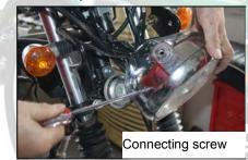
• Pull off the headlamp patch plug to remove the
