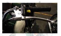
7) Adjust clutch and check clutch whether it declutch.
