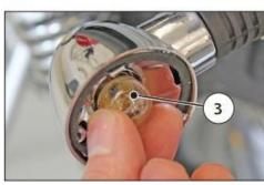
Position lamp bulb specifications: 12V5W
