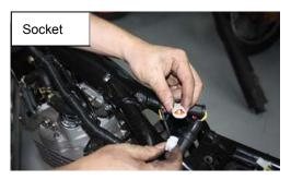
Dismantle rectifier bolt and measure two yellow wire whether is short circuit or broken circuit by millimeter.
