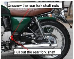
Remove the rear shock absorber and rear fork connecting
