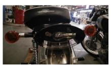
7. Check tail lamp and brake lamp socket whether lose
