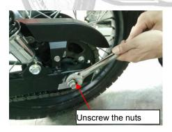
5) Remove the chain link and remove the drive chain.
