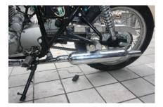
Remove the exhaust pipe
