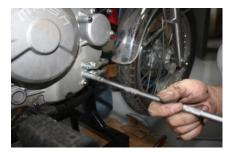
6) Adjust the direction of the clutch operating lever, Mount
