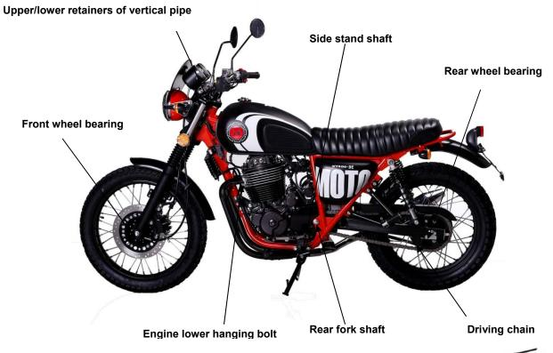
Among the positions shown in the above diagram, besides applying dedicated lubricating oil for chain to the driving chain, apply lithium base grease to all other positions.
