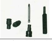
A and B bolt socket: for mantling/dismantling A and B bolt and exhaust muffler bolt
