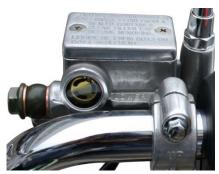
3) Actuate the brake handle, exhaust the air in the dead corner of the brake caliper.
