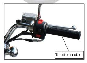
Take out throttle cable and check it whether is worn and fill lubrication oil.
