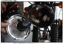
Pull off the left/ right turn lamp connecting wire from the headlamp bracket.
