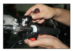
12. Check switch plug of relay whether is loose.
