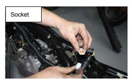
Dismantle rectifier bolt and measure two yellow wire whether is short circuit or broken circuit by millimeter.
