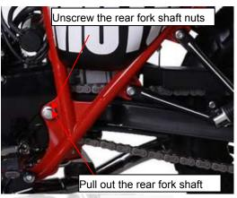
3. Remove the rear shock absorber and rear fork connecting
