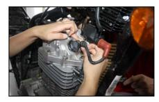
11. Remove the magnetic motor, gear display line and hit
