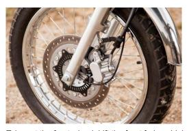
Take out the front wheel. Lift the front fork as high as possible while taking out the front wheel, to avoid damaging the front mudguard.
