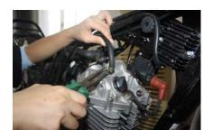
3) Remove Left /Right cylinder head connecting pipe
