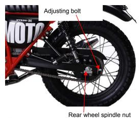
The scale lines of the chain adjuster on both sides must be consistent with each other.
