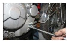
3. Remove side cover, seat and fuel tank
