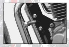
Dismantle the suspension bolt on the muffler, check whether it is sliding.
