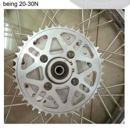
Take out bush and dismantle bolt of rear driven chain disc.
