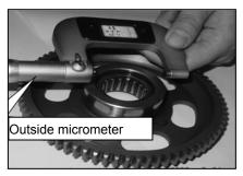
7) Measure the washer thickness, the maintenance limit:
