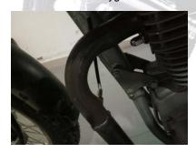
Remove muffler barrel body
