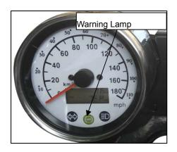
When the speed of the front and rear wheels difference greatly under extreme driving conditions, for example, the front wheel off the ground to performance the balance stunt or rear wheel slip, ABS warning lamp goes on, the ABS will fail. In order to reactivate the ABS, riders need to stop and close the ignition switch. If you restart the vehicle, ABS will restart.
