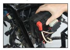
3. Check charging coil of magneto whether is charged.
