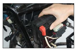
check connector socket of rectifier and measure output voltage by multimeter to (13.0-13.3)v
