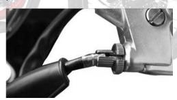
7) Adjust clutch and check clutch whether it declutch.
