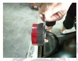
2. Check tail lamp and brake lamp socket whether lose
