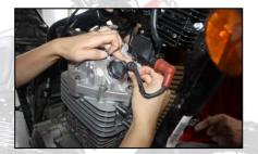
5) Unclamp the inlet pipe clip and remove the cylinder head hanging bolt.
