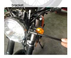
Remove the 2 connecting screw in the front face of the motorcycle.
