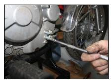
Remove the oil drain plug to drain the engine oil inside the crankcase.
