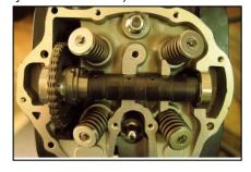
Remove the camshaft end cover, loosen the screw and washer at the tail end of the tensioner; turn the screw clockwise with the tensioner locking key
