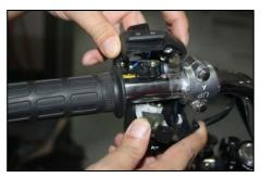
Check steering signal indication lamp socket whether lose contact or bulb is burned
