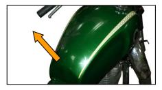
To avoid fuel line contamination, clog the joint with fireproof fabric after pulling off the fuel tube.
