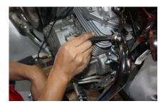
2) Remove the engine cycle tube
