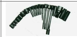
Socket: for mantling/dismantling nuts and bolts
