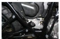
Pull out and pull off the patch plug of the rear brake lamp switch, and carefully pull out the rear brake lamp switch wire and remove the rear brake spring. Replace with new rear
