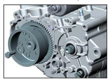
3) Mount the plain washer and apply thread retaining adhesive LOCTITE648 to the fastening nut M12; use the rotor fastening tool asten the rotor, and screw up the nut M12 to the torque of 45N.m
