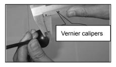
Measure the free length of the valve spring
