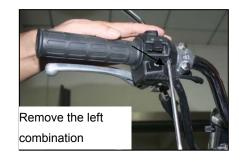
Loosen the retaining bolt and remove the clutch handle holder.
