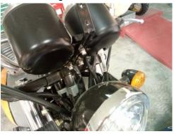
Take off meter to check odometer, tachometer and fuel meter whether are damaged.
