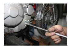
6) Adjust the direction of the clutch operating lever, Mount the clutch operating lever, rear brake return spring, cotter pin, rear brake lamp switch, etc.
