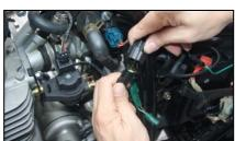
15. Remove the inlet pipe connected to the engine bolt
