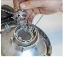
Position lamp bulb specifications: 12V5W
