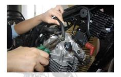
6. Remove Left /Right cylinder head connecting pipe
