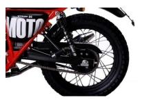
• Loosen the nut and remove the lower hanging bolt.
