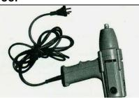
Motorized gun: special power tool for mantling/ dismantling bolt and nut
