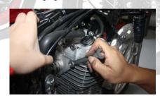
6) Remove the cylinder bolt and washer.
