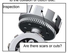
2) Check the clutch disc. If there is a scratch or de pigment or a strong scorching smell, replace it. Measure the thickness of each clutch disc.
