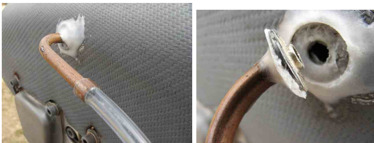
Figure 61: Ram Air duct pressure tapping.
