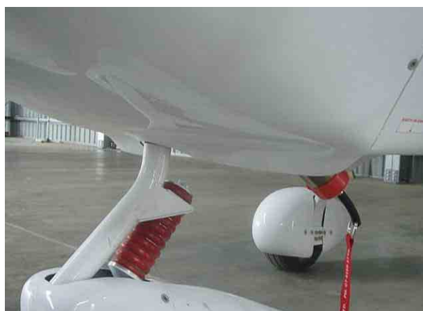
Figure 56: Lip to aid cooling as installed on a Jabiru.
