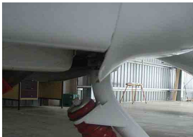
Figure 56: Lip to aid cooling as installed on a Jabiru.
